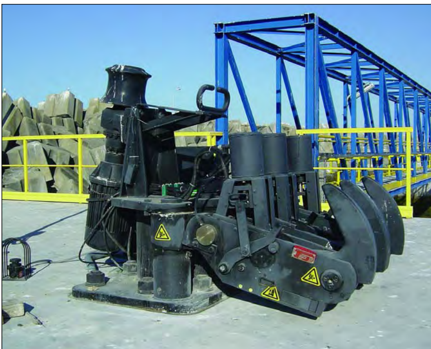
Mooring Hooks with Electric Solenoids (magnets)
