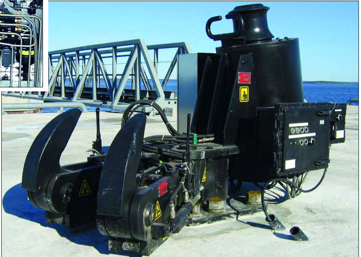
Mooring Hook Unit with Hydraulic Remote Control (suitable for -32° C operation)
