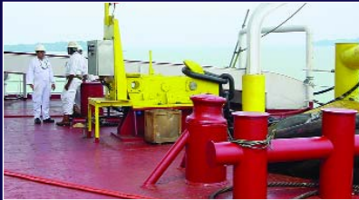
Hooks for FPSO's/FSO's executed as fixed or swiveling design. The hooks can be equipped with Remote Control Operation and Load Monitoring System. Standard execution from 200 up to 350 Tonnes S.W.L.
