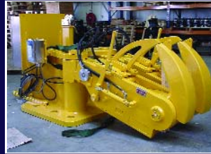
Hooks for FPSO's/FSO's executed as fixed or swiveling design. The hooks can be equipped with Remote Control Operation and Load Monitoring System. Standard execution from 200 up to 350 Tonnes S.W.L.
